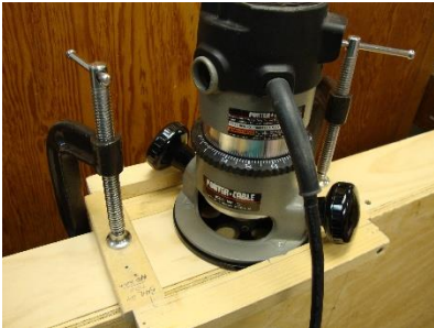
Figure 6 – Router in jig
