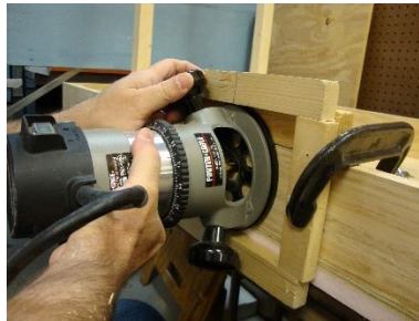
Figure 7 – Router making cavity
